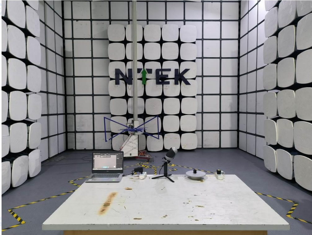
Radiated Measurement Photo
